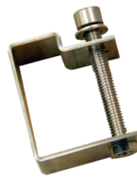
C clip Joining of two unsupported ends of adjacent panels
