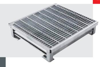
Surcharge Pit Grates are manufactured in a range of standard sizes and are hinged and bolted down with options for bolt down or cast-in legs, generally 300mm long. The bolt down range is suitable for existing pits or where the concrete has been poured before the grate arrives and bolted down to the pit surface wall as required. Cast-in legs are typically used when the grate is cast-in while the pit concrete wall is being poured.
