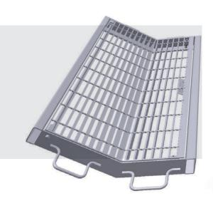
These grates are specifically designed to suit the roll of the kerb and are used predominantly in sub-divisions. All grates are hinged for easy access and bolted down to deter unwanted access. The frame comes with reo concrete tie-ins for easy tying into your formwork prior to casting. These grates meet the respective load class requirements of AS 3996:2019 as detailed in the table below.
